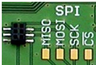
Figure 30: Wiring fields for SPI
